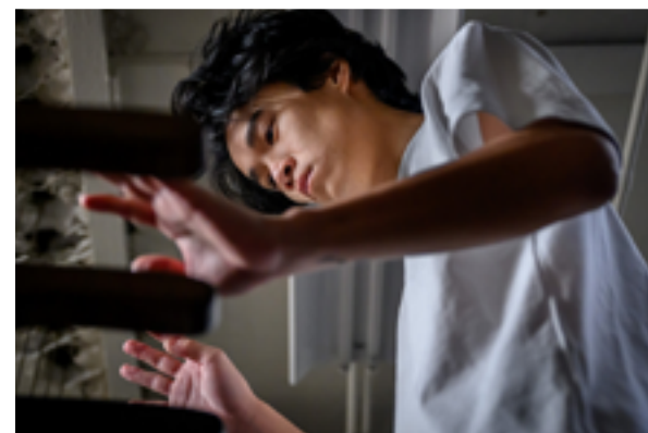
Each player has a different style of interacting with the levers that pull a cable to sound the chimes. Joseph Kim releases the key-like levers to let the bells ring. Photo: Fred Zwicky
