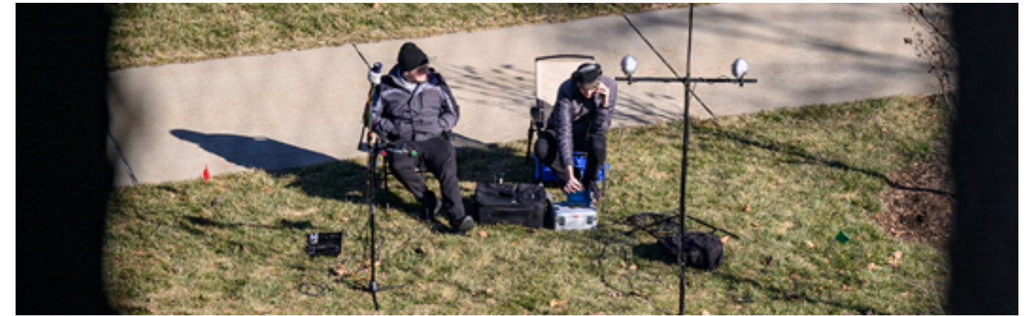
Sound engineer Graham Duncan and his assistant use several microphone pairs to record the chimes as they ring over campus, while navigating wind gusts and the sound of passing vehicles. | Photo: Fred Zwicky
